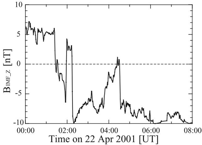
**Figure 2.** The 1-min interval data set of the IMF  $B_z$  component (in GSM coordinates) on 22 April 2001 measured by the MAG instrument onboard the ACE satellite. We have compensated the arrival time of every IMF at the average magnetopause ( $10 R_E$ ) from the ACE position ( $\sim 213 R_E$ ), taking into account the variation of the solar wind velocity.
