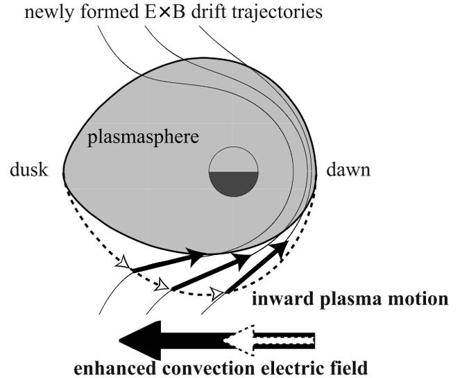
**Figure 4.** A schematic diagram of the inward plasma motion at the nightside plasmopause, in the convection electric field enhanced by the southward turning of the IMF. The dashed line indicates the previously formed plasmopause at the nightside. After the enhancement, the plasmas on the previous plasmopause move inward as black arrows along the newly formed  $E \times B$  drift trajectories.
