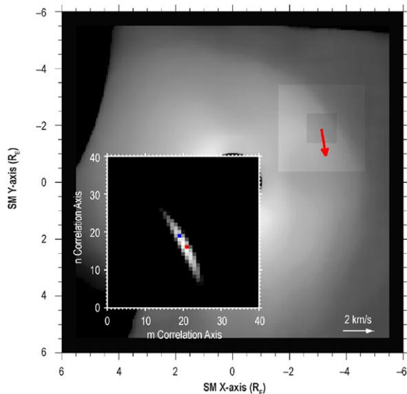
Fig. 4. The flow vector at 0555 UT and solar magnetic  $(x, y) = (-3.1, -1.9)R_E$  is shown in red. The shading around the arrow indicates the kernel size and the region across which the correlation analysis is performed. The graphic insert shows the correlation values below 0.01 in reverse gray scale, where the best value location is indicated by the red dot. The blue dot indicates that location along the ridge where the smallest drift velocity is located.
